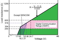
Figure 2 Supply Voltage and Load Resistance for ISC and pH/ORP SENCOM sensor
